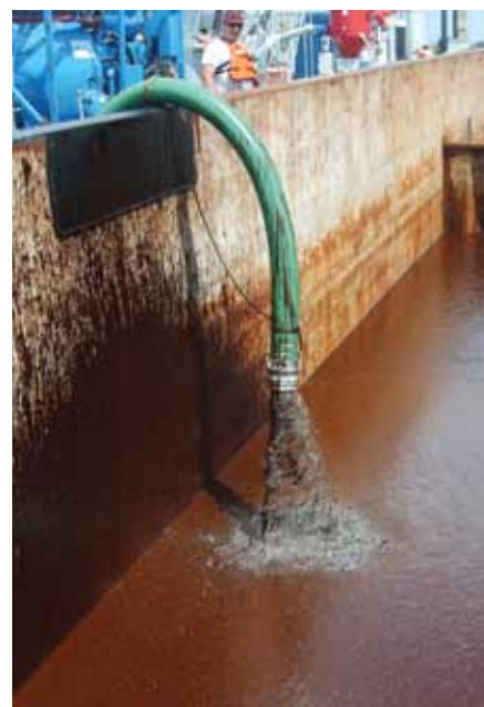
This photo shows oil collected by skimmer boats being transferred to an open hopper barge for transport to Beaumont, TX, for offloading. PSC tankermen have supervised many transfers like this in the Gulf since the April 21st rig explosion.
