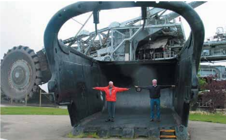
Cordell and Brian Haymon stand in a giant bucket used to mine oil sands near Fort McMurray, Alberta. In the background is an excavator more than 400 feet long.
